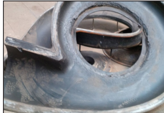
Damaged liner removed from casing
